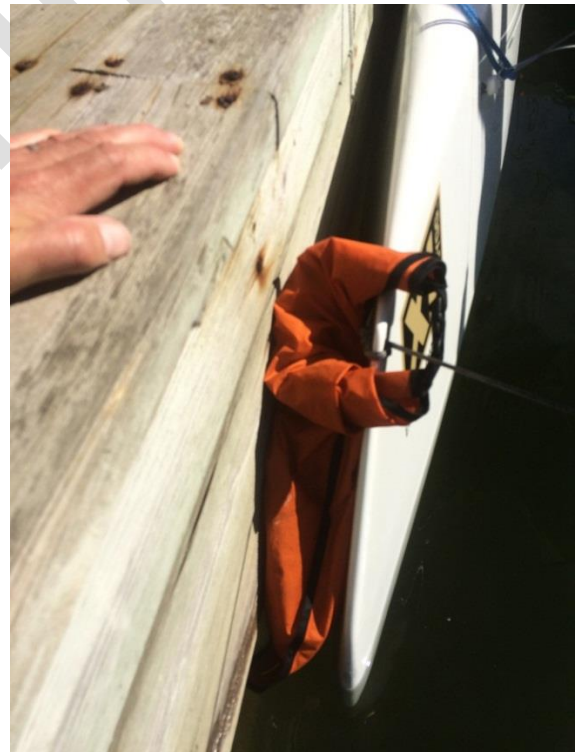
Figure 2 Waterproof bags in hulls for extra clothes can also be used as fenders at the jetty when boats are left in water over night
